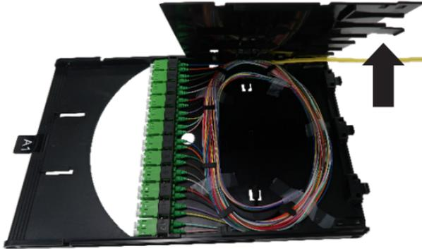
3. Splice the desired pigtail with the fiber drop cable in accordance with standard industry splicing practices.
