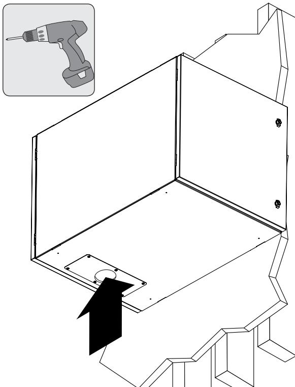
**Note:** This conduit cover supports a maximum Conduit Trade Size 2 with 2.5" hole.
