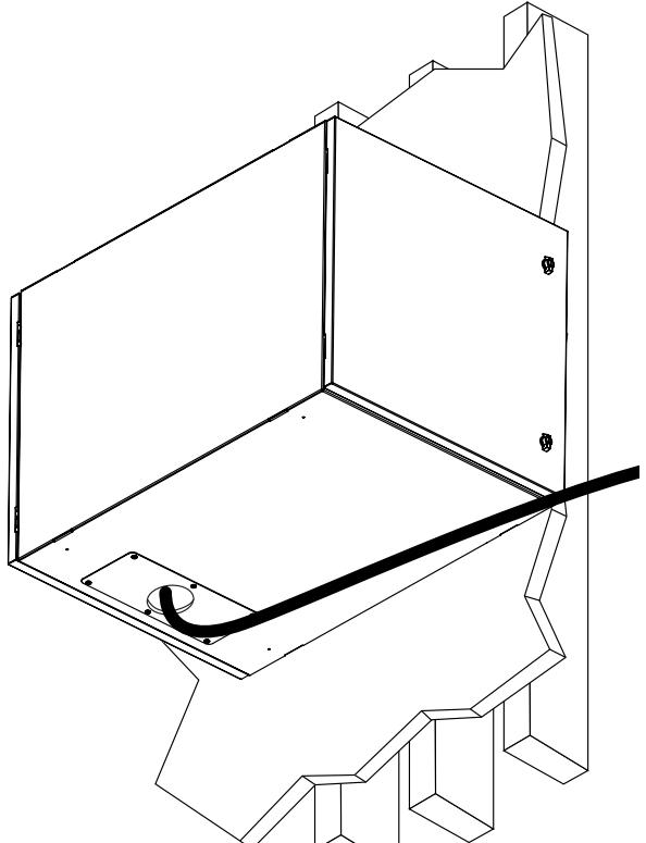
**Note:** To maintain a NEMA rating, use sealed fittings in the cutouts when connecting to conduit.
