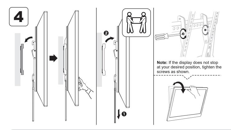
Using an assistant or mechanical lifting equipment, hook the display with attached adapter brackets over the top of the mounted wall-plate. Tighten the two screws of the adapter brackets to secure the unit.
