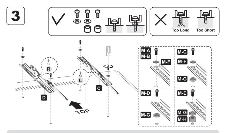
Note: Choose appropriate screws, washers and spacers (if necessary) according to the type of screen.
