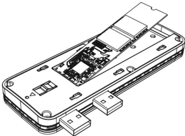
3. Gently press down on the M.2 SSD, and snap it into the standard rubber cartridge.
