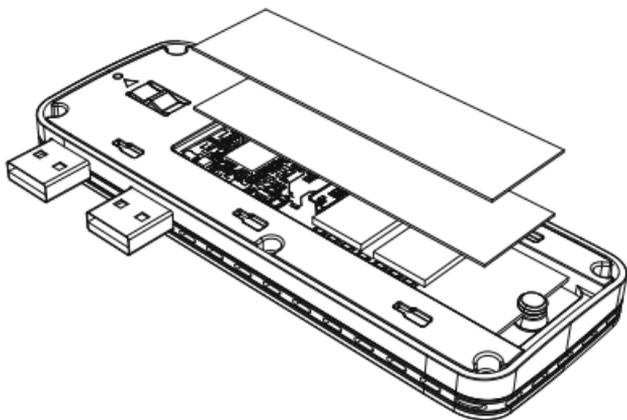
5. Attach the upper cover to the enclosure by pressing it and sliding it to the right.
