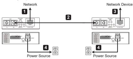
1 Connect the RJ45 port on the media converter to your network with a user-supplied Cat5e/6 cable.
