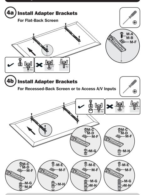
**Note:** Choose appropriate screws, washers and spacers (if necessary) according to the type of screen.
