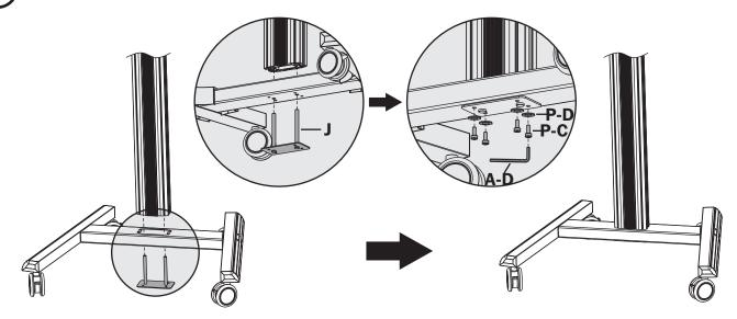
Insert the connecting piece (**J**) into the column to attach the column to the base. Use M8x35 screws (**P-C**), D8 washers (**P-D**) and the 6 mm hex key (**A-D**) to secure the connecting piece and column to the base.
