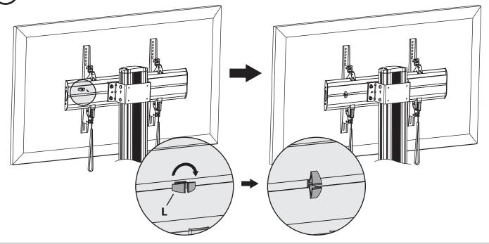
Insert the cable clamps (L) horizontally into the universal plates' slots, then turn the cable clamps vertically to secure them.
