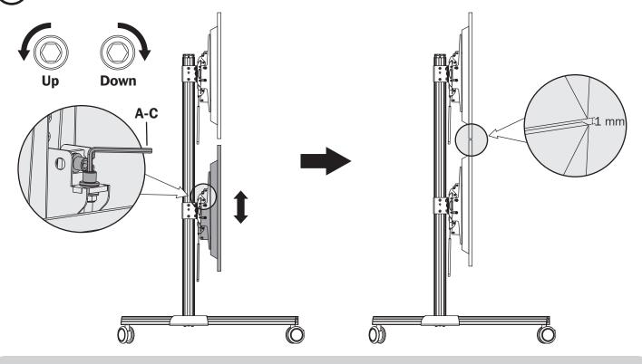
To move the displays up or down, adjust using the 5 mm hex key (A-C), as shown above.
