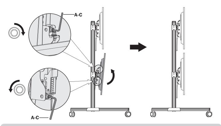
If the display tilts downward, adjust using the 5 mm hex key (A-C), as shown above.
