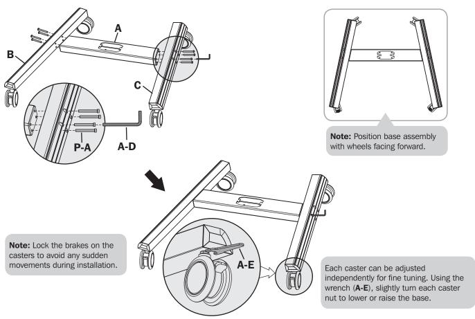
Using M8x65 screws (P-A) and the 6 mm hex key (A-D), attach the left and right base to the middle base.
