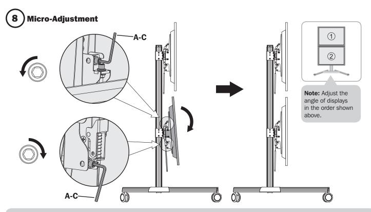
If the display tilts upward, adjust using the 5 mm hex key (A-C), as shown above.
