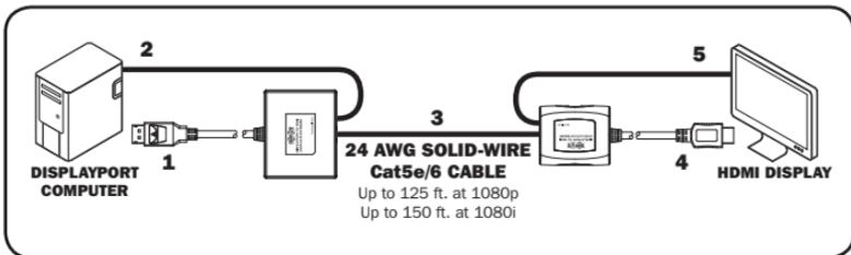
1. Connect the transmitter unit's built-in DisplayPort cable to the computer's DisplayPort output port.
