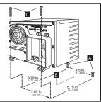
The polycarbonate cabinet and mounting feet of your Inverter/Charger are durable enough to allow for wall mounting as well (if your vehicle compartment requires this configuration). For wall mounting, the control panel of the Inverter/Charger must face to the side and not up or down.
