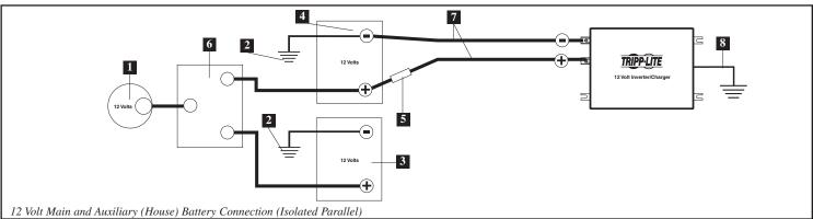
1 12 Volt Alternator 2 Vehicle Battery Ground 3 12 Volt Main Battery 4 12 Volt Auxiliary (House) Battery 5 UL-Listed Fuse & Fuse Block (mounted within 18 inches of the battery) 6 Battery Isolator 7 Large Diameter Cabling, Maximum 2/0 Gauge to Fit Terminals 8 8 AWG (minimum) Ground Wire
