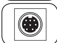
**PS/2 Port:** Use this port to connect a Tripp Lite ENVIROSENSE environmental sensor to provide remote temperature/humidity monitoring and a dry contact interface to control and monitor alarm, security and telecom devices. Visit [www.tripplite.com](http://www.tripplite.com) for ordering information. Note: *Do not connect a keyboard or mouse to this port.*
