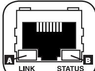
**Ethernet Port:** Use this RJ-45 jack to connect the PDU to the network with a standard Ethernet patch cable. The Link LED **A** and Status LED **B** indicate several operating conditions, as shown in the table below. *This port is not compatible with PoE (Power Over Ethernet) applications.*
