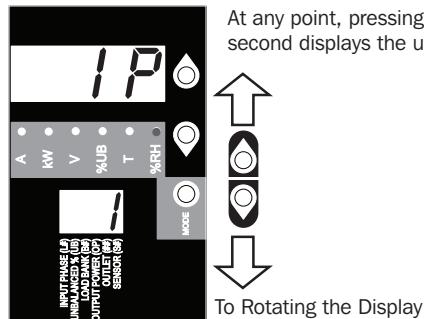
At any point, pressing both of the arrow buttons simultaneously for 1/2 second displays the unit's IP address in the 2-digit display.
