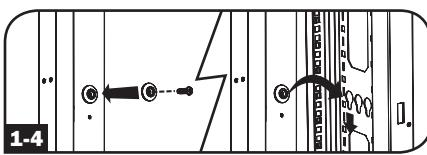
Note: Be sure to insert the 2 buttons into either the upper hole at **each end** of the PDU or into the lower hole at **each end** of the PDU.
