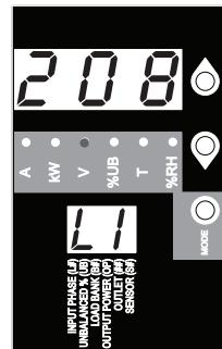
\*Note: For 208V models, voltages displayed are phase-to-phase voltages (i.e., L1 display will indicate L1-L2 voltage). For 400V models, voltages displayed are phase-to-neutral voltages (i.e., L1 display will indicate L1-N voltage).
