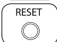
**SNMP Reset Button:** Press the reset button for 3 seconds to reboot the PDU's network card. Rebooting the network card will not erase network settings or interrupt AC power. The reset button is recessed. Use a paper clip or other suitable object to press it.
