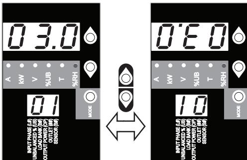
At any point, pressing both of the arrow buttons simultaneously and holding for 3 seconds rotates the 2-digit and 3-digit displays.
