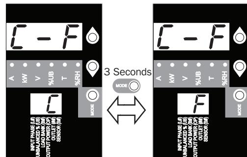
Hold Mode button for 3 seconds to switch between options. The letter in the 2-digit display indicates the selected unit, C for Celsius and F for Fahrenheit.
