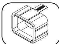
**C20 Plug Sleeve:** (Optional) Use the included C20 plastic sleeves to secure plugs to receptacles. Attach the sleeve to the plug making sure that the pull tabs remain outside the plug and that the fit is secure. To unplug equipment properly, use the pull tabs to remove the plug and sleeve from the receptacle.
