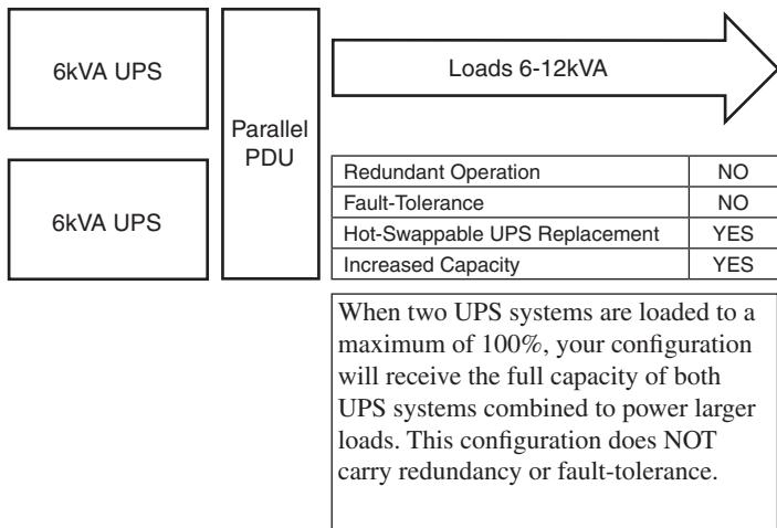
To ensure fault-tolerance, load the two parallel UPS systems to a maximum of 50% of the combined rating for both UPS systems. For example, if you have two 6kVA UPS systems, you will have fault-tolerant operation if the load level remains at 6kVA or lower.
