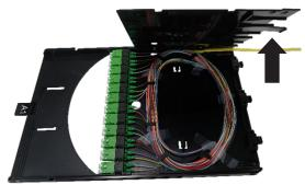
3. Splice the desired pigtail with the fiber drop cable in accordance with standard industry splicing practices.
