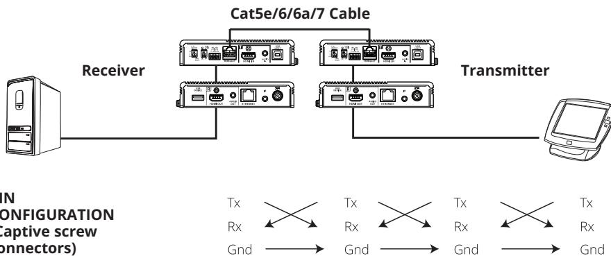
The general concept here is that an RS-232 signal can be transmitted (Tx) to the receiving (Rx) end of a unit. The received signal can then be transmitted (Tx) to the receiving (Rx) end of another unit. The RS-232 signals can be transmitted back the other way.
