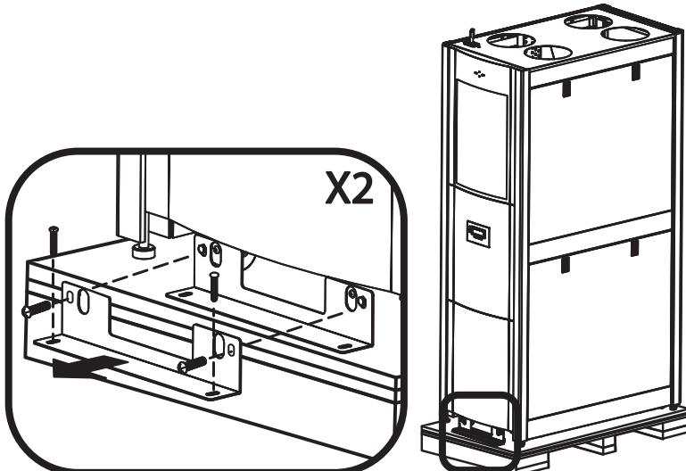
**5** Attach ramps to pallet. Insert ramp mounting tabs into mounting groove on pallet. Position ramps so they are aligned with the unit's wheels. For added safety, Tripp Lite recommends you secure the ramps to the pallet with user-supplied screws.
