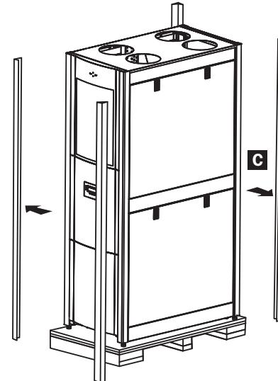
**3** Confirm that the model name and rating at the rear of the cabinet match the unit you ordered. Examine the cabinet for any damaged parts. The container should include the unit's Installation Manual, Owner's Manual and four Air Ducts.
