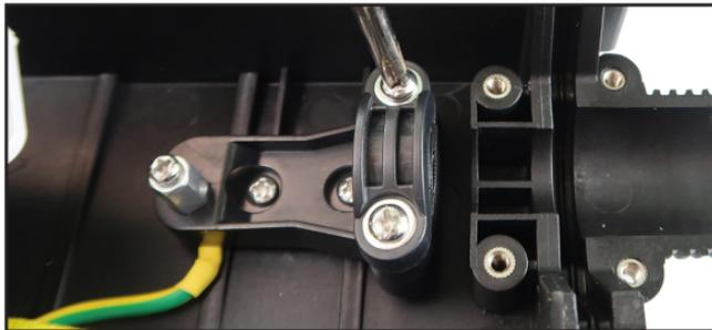
Figure 1-23: Remove the press clamping
