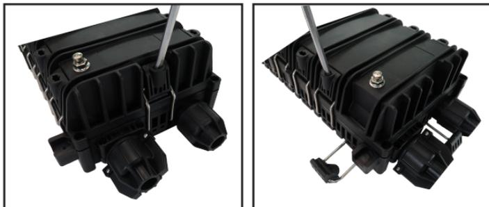
Figure 1-1: Open the buckle of the closure
