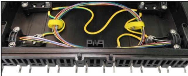
Figure 1-16: Install the pass-through cable on the other side
