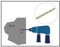
Figure 2-5: Drill holes in the wall
