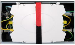
Figure 1-19: Close the splicing tray cover
