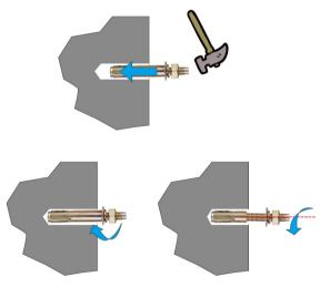
Figure 2-7: Install the expansion bolt
